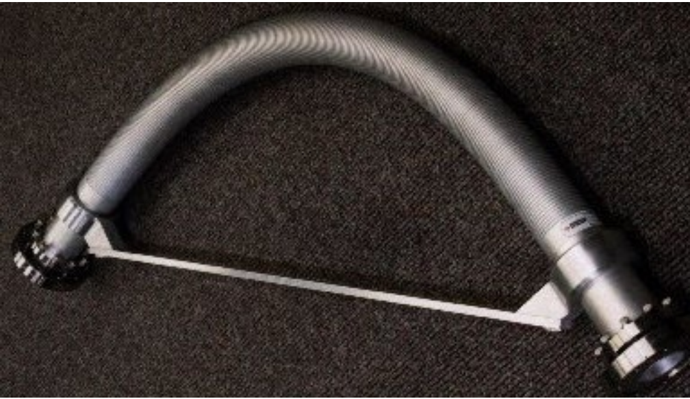
General Atomics high power 90° profilled curvature bend in 44.5 mm corrugated waveguide for TE_{01} mode at 11.424 GHz
